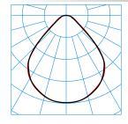
Belviso D CDP LED3900nw ETDD +LLWRC 01 TX064395 C0 - C180 UGR I = 16.2 UGR q = 16.2 UGR q = 16.3 DIN 5040: A50 UTE: 1,00 C DLOR: 99 % ULOR: 1 % CEN Flux Code: 66 90 97 99 100 17 42 75 1
