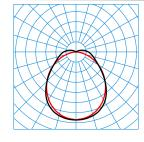
OleveonF 15 L 6000-840 ETDD PC+LLWRC LV TX056147 UGR I = 23.0 UGR q = 24.2 DIN 5040: A40 UTE: 0,94 E + 0,06 T DLOR: 94 % ULOR: 6 % CEN Flux Code: 47 76 92 94 100 4 9 34 6
